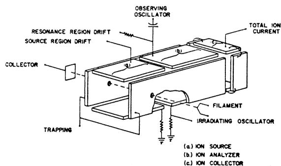
Fig. 1. Schematic diagram of the ion cyclotron resonance drift cell. (a) Ion source; (b) ion analyzer; and (c) ion collector (reprinted from [58]).
